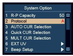
c) User can choose SCAN COIN protocol (A) or the protocol specific for SC 8220 CashNetwork software (B) by using the navigation keys.
