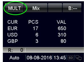
The machine can process three currencies simultaneously.
