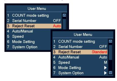
With "Auto" activated, the machine clears the reject number automatically as soon as the banknotes are removed from the reject pocket, even while the machine is still counting.
