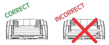
**d)** Adjust the note guides according to the longest banknote in the stack.
