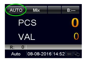
The machine recognizes the currency according to the first note, provided that the currency is ON in the AUTO CUR Selection menu.
